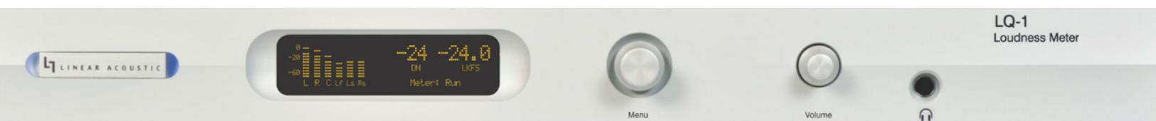
Comprehensive SDI, AES, Optical, Analogue and DVB-ASI inputs followed by decoding for PCM or Dolby encoded audio, then loudness measurement per ITU-R BS.1770 with selectable Dolby Dialogue Intelligence automatic gating. The result is a metered value that agrees with standards and recommended practices such as ATSC A/85 and EBU R128 as well as accurately reflecting listener perception.
